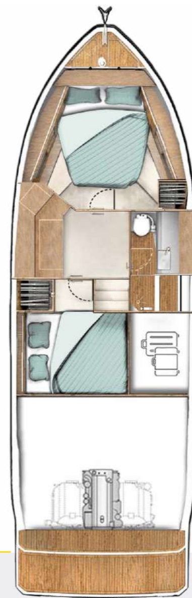
LOWER DECK standard with storage space midships
